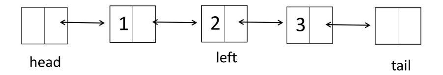
Suppose *left* is pointing at the box with datum 2. We are saying this is to the left of our logical position, so our actual location is between box 2 and box 3. On a call to next we move to the right and return 3. Here is code that achieves this:
